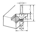
CARBIDE TIPPED - Ball Bearing Pilot
